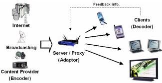
Fig. 1. Role of adaptor in scalable video coding application.
